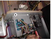
3. Assemble new chute assembly @ using (8) supplied screws and nuts.
