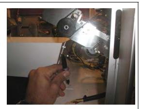
5. Using the marks, pre-drill mount screw holes using a 1/8" drill bit.
