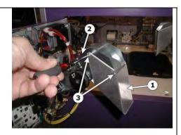
2. Remove inside most <u>power supply mount</u> <u>screw</u> from the <u>ticket basket plate</u>. Insert the supplied #12 x 5/8" screw in its place from the bottom.
