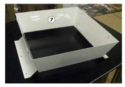
4. Place the <a href="mailto:new chute assembly">new chute assembly</a> on the <a href="mailto:new chute should be">ticket basket plate</a> inside the machine. The chute should be approximately centered from left to right and from front to back. Use the ticket chute as a template to mark the ticket basket plate mount hole locations. Use the side doors for easier access.
