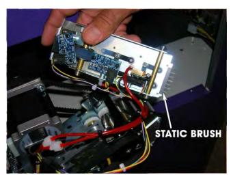
Remove Top Assembly Clean rear top edge of sheet metal where static brush will mount. Adhere static brush along back edge of top assembly between rivets as shown. See manual or inside front door for instructions.
