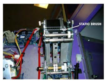
Clean sheet metal on bottom side of ticket taker at back edge where static brush will be installed.
