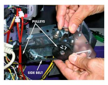
Remove side belt by loosening both pulley clamps and pulling both pulleys off of the shafts simultaneously.
